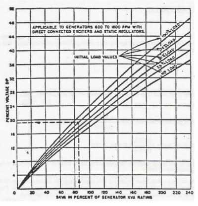
Voltage Dip with Motor Starting Loads
