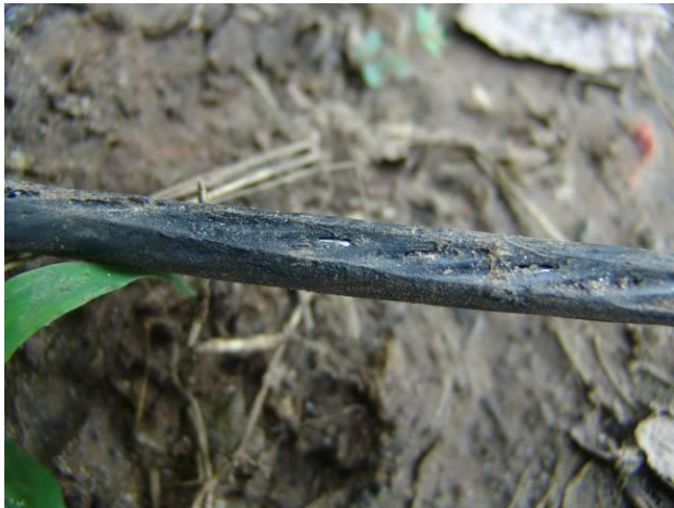
Figure 4: Damage from overheated neutral
